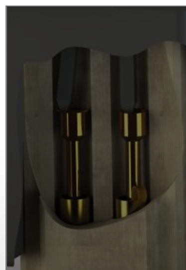
Abrasion/dirt = Spring contact pins' service life massively reduced = Plug's shape/tolerance not OK
