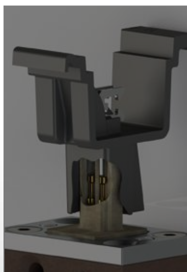
Not OK contact pins = abrasion/dirt
