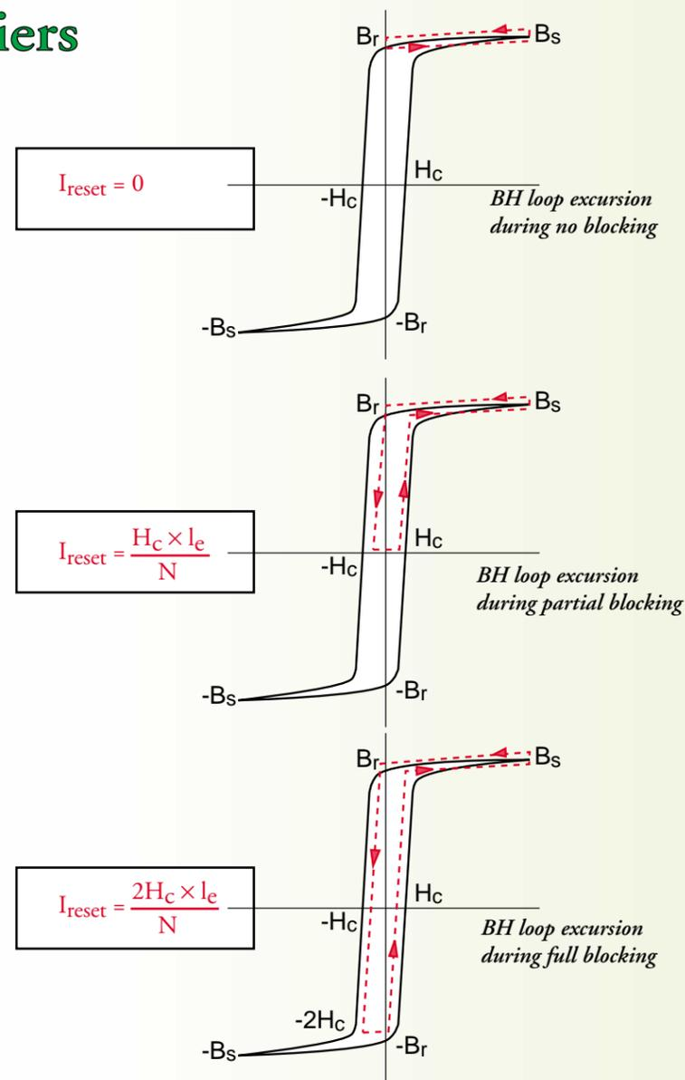
$$I_{\text{reset}} = \frac{H_c \times l_e}{B_r \times N} \times \Delta B$$
