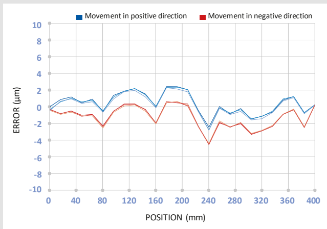
Repeatability graph obtained by carrying out the measurements several times in both directions of advancement.
